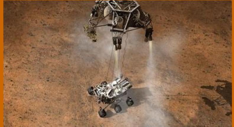
• Curiosity is tasked with collecting rock and soil samples and placing them into onboard instruments for analysis. With this in mind, the rover comes equipped with a 2.1-meter camera mast and a 2-meter, three-jointed robotic arm which can scoop, dust, drill, powder, collect, sort, sieve and deliver samples.
